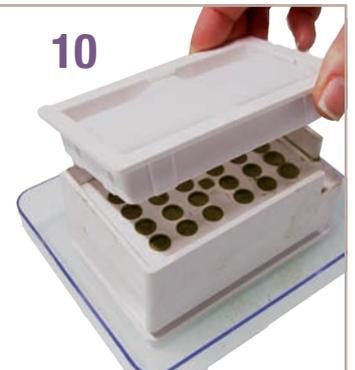
10. Place the high part **3** of the machine on the low part **2**.
